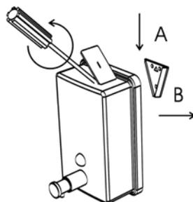
1. Unscrew the set screw inside the back of dispenser, and take out the wall bracket
