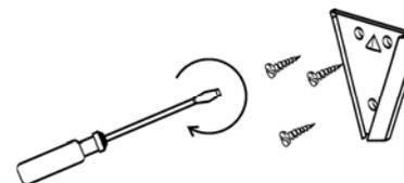
5. Install the wall bracket by screws
