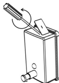
7. Tighten the set screw which inside the back of dispenser
