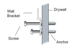
Place back of frame over top of wall bracket so that wall bracket slips between back of board and metal frame. Center the board on brackets.
