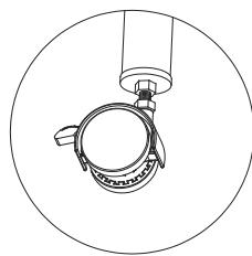
Make sure the gold hex nut is fully tightened around the black center pole
