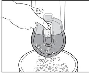
Hold dust cup over wastebasket and press lever to release bottom lid. Debris will empty.
