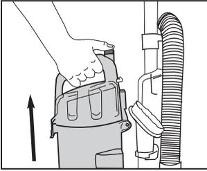
Press release button and lift off dust cup.
