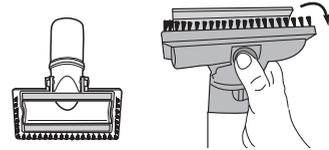
**2-in-1 upholstery tool (NEU188)** – Use brush to vacuum upholstered surfaces or pick up debris. Use felt portion to clean delicate surfaces. Press thumb release and lift brush up and out of the way.
