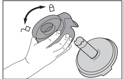
Grip tabs and lift out filter screen. Twist bottom of filter screen counterclockwise to unlock and pull apart. Shake off dust. Rinse screen and dust cup. Dry all THOROUGHLY. Reassemble screen; twist clockwise to lock.
