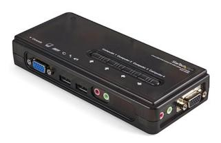
The SV411KUSB 4 Port USB KVM Switch Kit with Audio and Cables lets you control up to four USB-enabled computers using a single keyboard, mouse and VGA monitor and offers both hotkey and top panel push-button operation for simple switching between connected computers.
