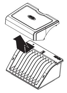
3 Lift and remove the storage shelf from the enclosure.
