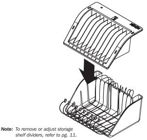
**E** Connect the electronic devices to the USB power cables and place items inside the shelf tray.
