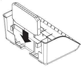
Connect USB charging cables appropriate for the number and type of devices. The slots located at the top and front of the enclosure base allow for convenient cable routing.
