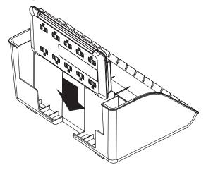
**B** Connect the AC power cables appropriate for the number and type of devices. The slots located at the top and front of the enclosure base allow for convenient cable routing.
